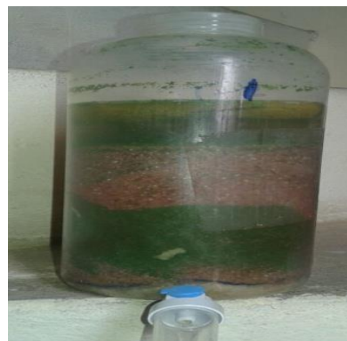
Fig 3 Neem leaf Powder Bottle Filter
